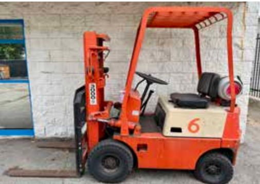
FORKLIFT TOYOTA, MODEL 2FG15, 3,000 LB CAPACITY, 3-STAGE MAST, LPG, LOAD LIGHTS, S/N 11511
