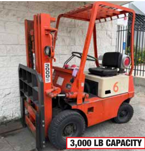
FORKLIFT TOYOTA, MODEL 2FG15, 3,000 LB CAPACITY, 3-STAGE MAST, LPG, LOAD LIGHTS, S/N 11511
