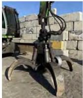
2020 SENNEBOGEN 830 M E-SERIES. **CUMMINS B6.7 DIESEL ENGINE,** 225 HP, 55'9" REACH, MAXCAB II ELEVATING CAB SYSTEM E270, K15 - REACH 50'3, STRAIGHT BOOM **27'11. END STOP MONITORING** SYSTEM AND LIMIT SWITCHES. STRAIGHT STICK 23', WITH END STOP MONITORING SYSTEM AND **LIMIT SWITCHES, RUBBER TIRES,** ALL WHEEL DRIVE, 4-POINT 9' **OUTRIGGERS, COMPUTER FREE.** STATE-OF-THE-ART LOAD-SENSING WITH FLOW-ON-DEMAND CONTROL, S/N 830.0.2962, STANDARD **MACHINE CONFIGURATION, CLAMSHELL GRAB ATTACHMENT**
