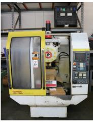
**FANUC DRILL MATE T MODEL 10, TRAVELS:** 19.6" X 14.9" X 12.9", 36" X 14" TABLE, 12.000 RPM SPINDLE, CAT 35 TAPER, 10 STATION ATC, 20 HP, FANUC OM CNC CONTROL, S/N T914TA078
