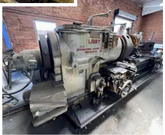
LIBBY H TYPE, 12" HOLE THRU, 24" X 84" CC, 28" 4-JAW CHUCK, 5-STATION TURRET, 1,800 RPM SPINDLE SPEED
