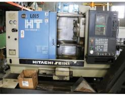
1999 HITACHI SEIKI MODEL HT23J, SEICOS J CNC CONTROL, 8" Chuck, 4,500 RPM, 2.5" BAR CAPACITY, TAILSTOCK, Mayfram Chip Conveyer, S/N Htj3787hl, CNC Enhancements Autobar 400 Bar Loader
