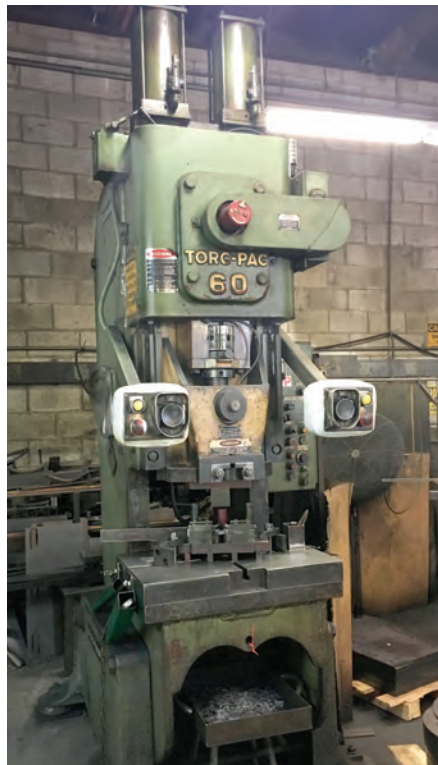
CLEARING TORMAC OBI, MODEL 60T-701, 60 TON, 90 SPM, S/N 85-1282-14
