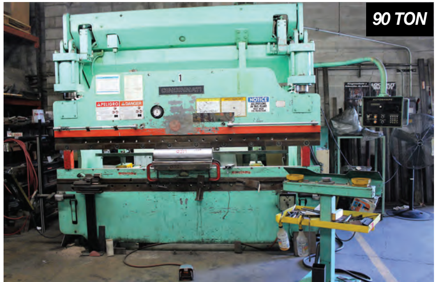
CINCINNATI AUTOSHAPES CNC HYDRAULIC PRESS BRAKE, MODEL 90 AS 8, 10' X 90-TON CAPACITY, 8'6" BETWEEN HOUSING, 8" MAX STROKE, AUTOSHAPES CNC BACK GAGE, PROTECH EAGLE EYE PROTECTION, S/N 43355
