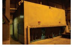
ENCLOSURE WITH APPROX. 150' -36" ROLLER CONVEYOR, SCISSOR LIFT TABLES, FOUR SIDE DRAFT EXHAUSTS, APPROX. 7000 CFM DUST COLLECTOR WITH BLOWER AND MOTOR, WELDERS AND HOISTS
