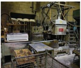
3- SHELL PROCESS OR SHALCO MODEL DSM 3 SHELL MOLDING MACHINES EACH EQUIPPED WITH UNIVERSAL FEED BUCKET ELEVATOR, DRIVE, MOTOR, HYDRAULIC SYSTEM, (2) OVENS, PICKOFF SYSTEM, GAS SYSTEM, CONTROLS AND EITHER (2) 1520 PIN BONDERS WITH GLUE APPLICATORS OR (1) 2030 PIN BONDER WITH GLUE APPLICATOR
