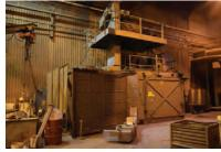
PANGBORN MODEL 12LK3 12' DIAMETER TABLAST SHOT CLEANING MACHINE WITH 3 BELT DRIVE SHOT WHEELS, SHOT SYSTEM AND CONTROLS
