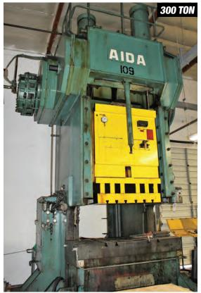
AIDA MODEL PC-30, 300 TON CAPACITY, AIR CUSHION, 15.7" STROKE, 30 SPM, 70" X 30" BOLSTER AREA, 45" X 30" SLIDE AREA, 4.7" SLIDE ADJUSTMENT, S/N 15000-0606
