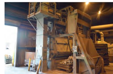
2007 PANGBORN MODEL 12LK3 12' DIAMETER TABLAST SHOT CLEANING MACHINE WITH 3 BELT DRIVE SHOT WHEELS, SHOT SYSTEM AND CONTROLS
