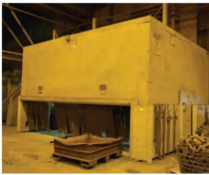
ENCLOSURE WITH APPROX. 150' -36" ROLLER CONVEYOR, SCISSOR LIFT TABLES, FOUR SIDE DRAFT EXHAUSTS, APPROX. 7000 CFM DUST COLLECTOR WITH BLOWER AND MOTOR, WELDERS AND HOISTS
