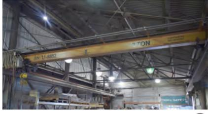
3 TON APPROX. 40' SPAN SINGLE GIRDER BRIDGE CRANE WITH GARDNER DENVER HOIST
