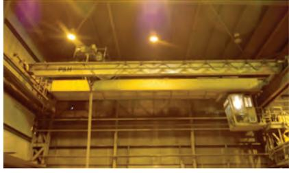
P AND H 15/5 TON OVERHEAD DOUBLE GIRDER TOP RUNNING BRIDGE CRANE, CAB OPERATED, 43' SPAN, 26' LIFT
