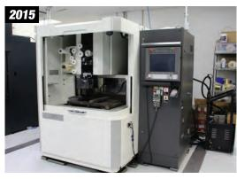
2015 MAKINO UPV-3, 3-AXIS, 24.8"X17.71" TABLE, TRAVELS: X-14.56", Y-10.63", Z-8.7", TANK SIZE 31.1"X24.05". NO DROP TANK. MAX. WORKPIECE WEIGHT 771 LBS., MAX. WORKPIECE SIZE 30.71"X 23.23"X3.94". OIL-BASED DIELECTRIC SYSTEM. MAKINO HYPER I CNC CONTROL, S/N E080471
