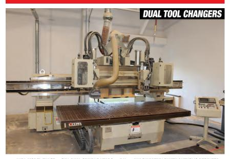
1998 ANDI, MODEL EXACT 51/MH, DUAL SPINDLE HEADS, 63" X 122" VACUUM TABLE WITH PHENOLIC RESIN TOP WITH POPUP STOPS, DUAL (12) STATION TOOL CHANGERS, SK-30 TOOL HOLDERS, 18,000 RPM, 10HP MOTOR, 25 HP VACUUM PUMP, FANUC 18-M CNC CONTROL, S/N 01-87049
