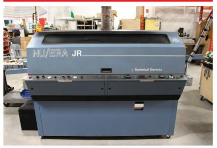
TECHNICAL DEVICES NU/ERA JR WAVE SOLDER MACHINE, LEAD FREE REBUILT TANK
