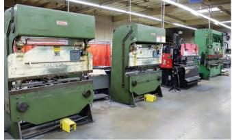
CINCINNATI 90 CB-8, HYDRAULIC 90 TON X 10' OVERALL, DISTANCE BETWEEN HOUSING: 8', 6.5", STROKE: 8", THROAT: 7", HURCO AUTOBEND 7 CNC BACK GAGE, S/N 42875
