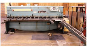
AMADA MODEL M-3045, 10' X 3/16" CAPACITY, MECHANICAL, 9' SQUARING ARM, (2) 31" SHEET SUPPORTS, AUTO REAR SHEET SUPPORTS, S/N 3045402
