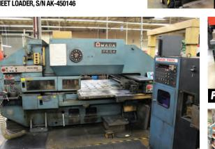
1981 AMADA PEGA 304040, 30 TON, AMADA FANUC CONTROL, 40" X 80" MAX. SHEET SIZE (WITH REPOSITIONING), 56 STATION, THICK TURRET, BALL TRANSFER TABLE, S/N AK-440009
