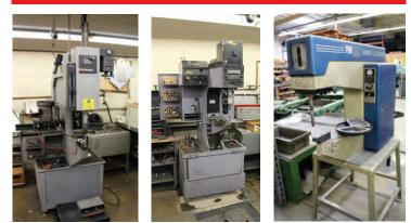
HAEGER 824, ADJUSTABLE UP TO 16,000-LBS. (72 KN) FORCE RANGE, 24" THROAT DEPTH, 0–8.5" ADJUSTABLE STROKE LENGTH, 1,500/HOUR INSERTIONS AT 1", 5 HP MOTOR, MODUALAR AUTOFEED SYSTEM, BATCH COUNTER
