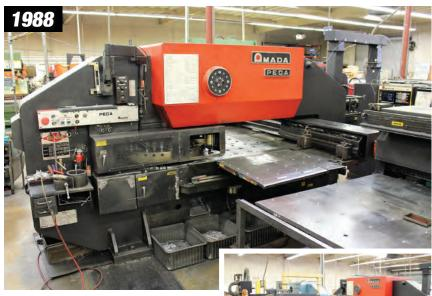
1988 AMADA PEGA 304050, 30-TON CAPACITY, 40" X 50" MAX. TRAVERSE, 40" X 100" MAX. SHEET SIZE (WITH REPOSITIONING), 350 STROKES PER MINUTE, 58-TOOL STATION TURRET, AUTO. INDEX CONFIGURATION, 60 RPM, 30 RPM TURRET SPEED, AMADA FANUC P SYSTEM 6M CNC CONTROL, 58 STATION THICK TURRET, HYDRAULIC CLUTCH AND BRAKE, BALL TRANSFER TABLE, AMADA SHEET LOADER, S/N AK-450146
