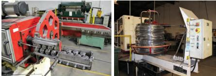
2001 LATOUR ROBOMAC MODEL 310 CNC 3D WIRE BENDERS; WIRE DIA. RANGE: .118" TO .393" (3 TO 10MM), FIVE AXIS, FORMING HEADS, FEED LENGTH UNLIMITED, (1) WITH REAR ROTATING STRAIGHTENING ATTACHMENT, DNC-800 CNC PROGRAMMABLE CONTROL, LATOUR MODEL D1000 MOTORIZED HORIZONTAL DECOILER; S/N 01-011-53
