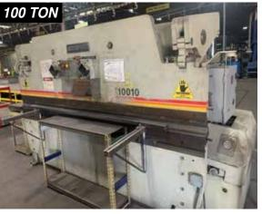
1997 ACCURPRESS MODEL 710010 HYDRAULIC PRESS BRAKE, S/N 4626; 100-TON X 10" CAP, 8' BH, CNC BACK GAGE
