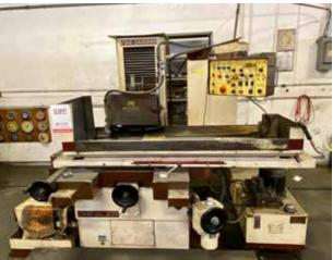
CHEVALIER FSG-1640AD, 3-AXIS, HYDRAULIC, 16" X 40" ELECTRO MAGNETIC CHUCK, AUTOMATIC INCREMENTAL DOWNFEED, S/N 485B002
