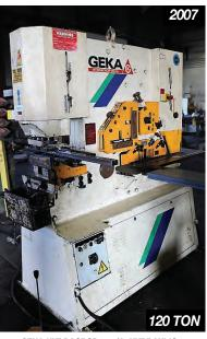
2007 GEKA HYDRACROP 110/A, HYDRAULIC, 120 TON, 12" PUNCH THROAT, 2" BAR SHEAR, 24" X 5/8" PLATE SHEAR, ASSORTED PUNCHES, S/N 21900
