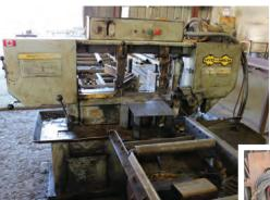
1995 HYMECH V-18, VERTICAL TILT, **18" X 21" CAPACITY** HYMECH S-20, HORIZONTAL. 13" X 18" CAPACITY, MITRE TO 45 DEGREES, 162" BLADE, S/N 20494750
