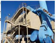
BAHNSON / HAWLEY NORFELT PULSE TYPE DUST COLLECTOR RATED AT 78,000 CFM WITH 200 HP DRIVE, MOTOR, NEW YORK SIZE 608III BLOWER S/N W-681-100 & CONTROLS BAHNSON / HAWLEY PULSE TYPE DUST COLLECTOR RATED AT 25,000 CFM WITH 125 HP **DRIVE, MOTOR, BLOWER & CONTROLS**
