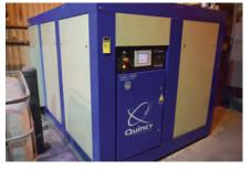
QUINCY MODEL QSI 1000 1000 CFM 300 HP WATER COOLED ROTARY SCREW TYPE AIR COMPRESSOR, DIGITAL READOUT
