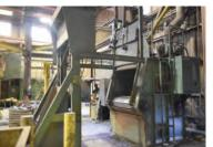
2007 PANGBORN MODEL 12LK3 12' DIAMETER TABLAST SHOT CLEANING MACHINE WITH 3 BELT DRIVE SHOT WHEELS, SHOT SYSTEM AND CONTROLS
